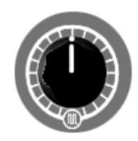
LOW FREQUENCY PULSEWAVE OSCILLATOR. USED TO STEP AND TRIGGER OTHER MODULES AT USER DEFINED RATE. ILLUMINATED ICON BELOW RATE KNOB INDICATES CLOCK PULSES. DESPITE THE LOCATION IN THE CENTER OF THE DECADE RING MODULES (DESCRIBED BELOW), THE CLOCKS ARE NOT NORMALLED TO THE DECADE RING MODULES. THEY ARE SEPARATE MODULES.
